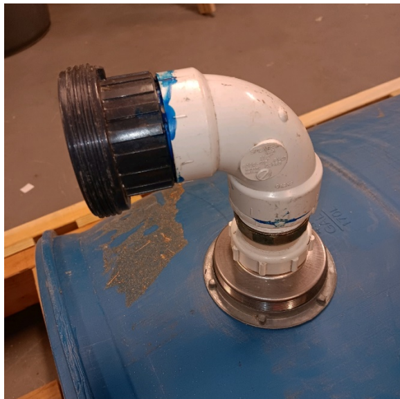
The removable bend glued to a 1-1/2" Union for removal and storage. A point close to one end of the basin is located say 4" away from the side from inside and marked. A sample hole tracing paper provided on the sink drain is measured and the right hole saw is used to cut the right hole at the marked location. If unsure, cardboard is first drilled with the hole to ascertain if it is the right size of the hole to fit the sink drain. The sink drain is fitted after the hole is made as in picture above. An
