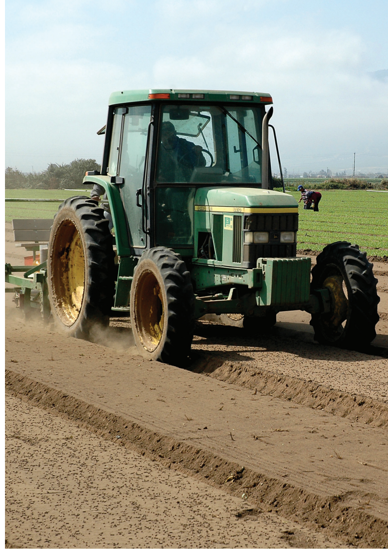
Heavy machinery can physically compact soil particles, reducing the pore space through which air, water, and nutrients flow and restricting root growth. Photo by Carlo Fanti
